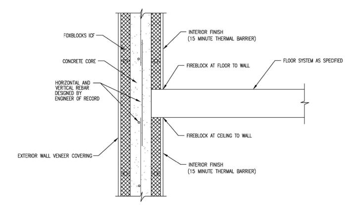
Figure 3 – Typical Wall-to-Floor Intersection for Types I, II, III and IV Construction
